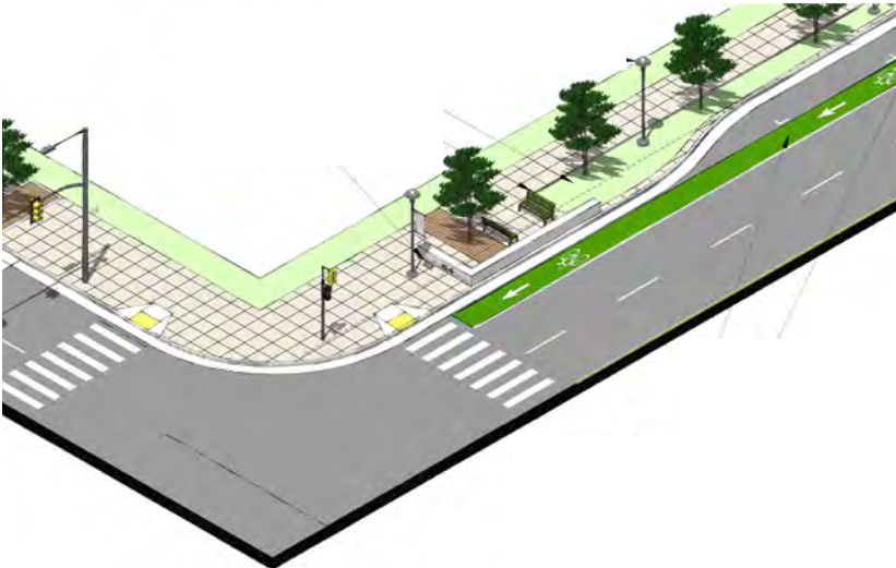
Figure 23: Illustrative Curb Bulbout if Bicycle Lane Present
